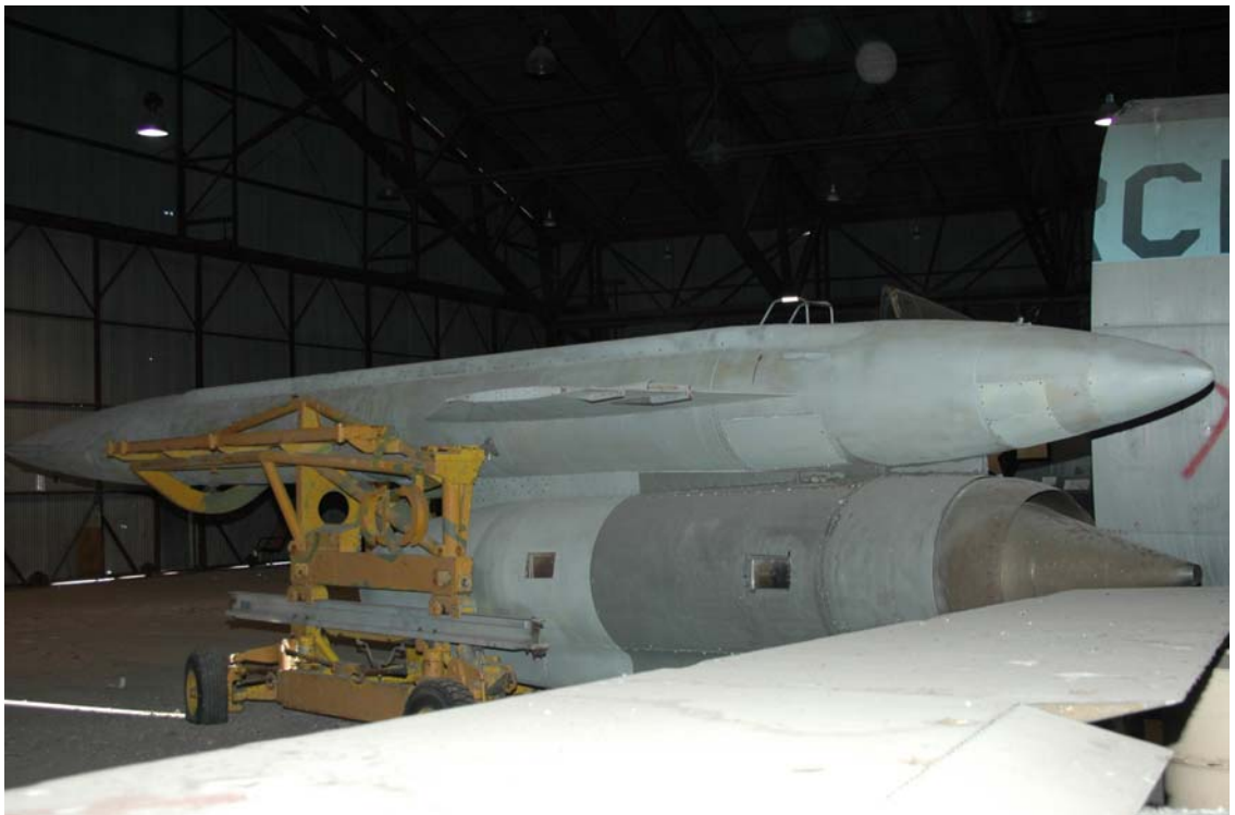
The Hound Dog seen from the port side rear. Note the underslung J52 rocket engine.
