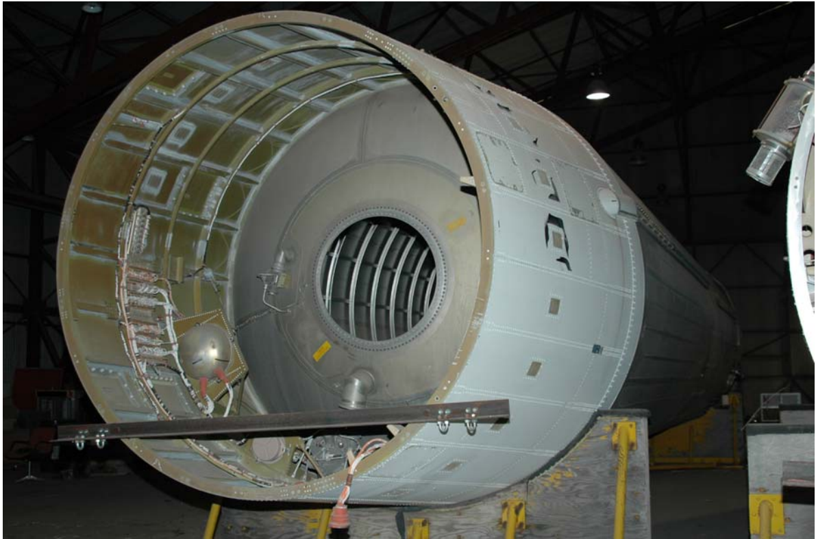
This is a view of the second stage where it would intersect with the reentry vehicle (warhead).
